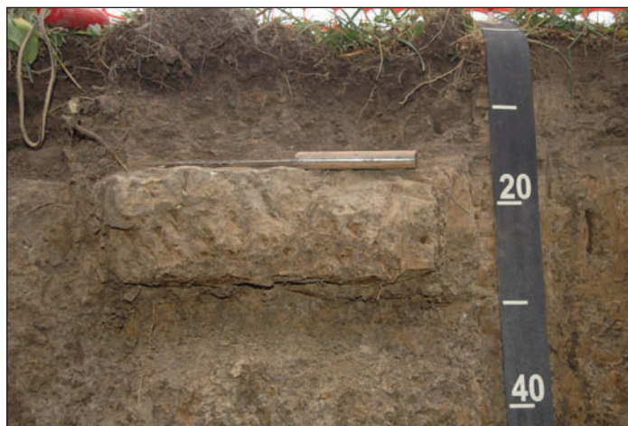
Image 2: Compacted layer (15 to 30 cm, or 6 to 12 inches) on urban soil research plot at The Morton Arboretum (Spring, 2007).
