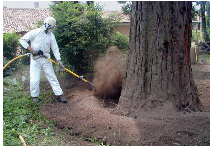
AirSpade being utilized for root collar excavation: Product development has gone hand-in hand with scientific research and the growth of practical applications in professional tree care services.
